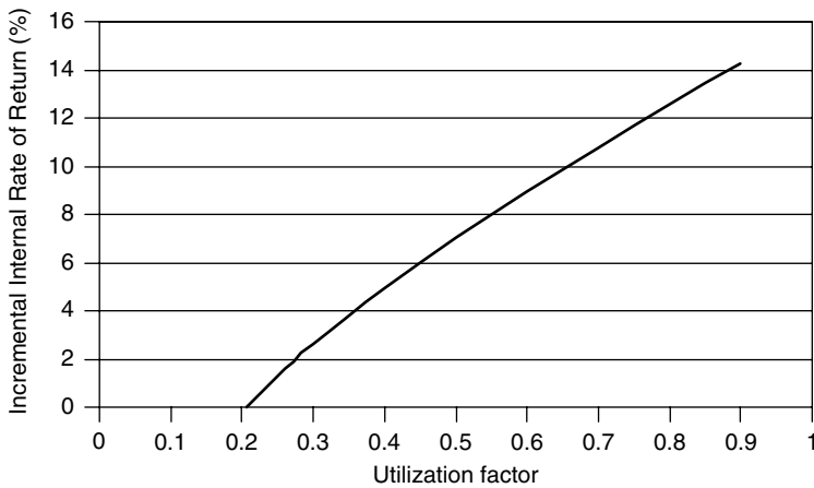
Figure 7.3 Incremental Internal Rate of Return that Borduria Power would achieve by investing in a coal plant rather than a CCGT plant
